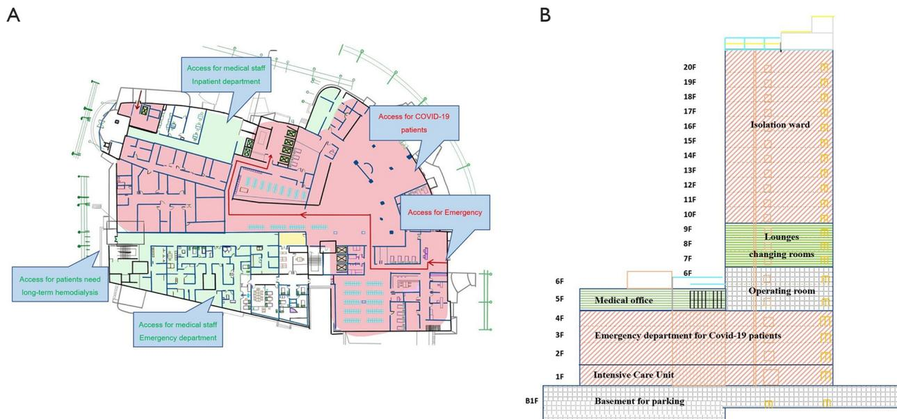
**Figure 1** Section distribution of Wuhan Third Hospital after reconstruction. (A) Section distribution of the main medical building. (B) Floor distribution of the main medical building. The green section means clean area, the red section means contaminated area and the grey section means closed area (drawn by Chunhui Xu).
