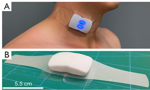
**Figure 1** The wireless Doppler ultrasound patch.
